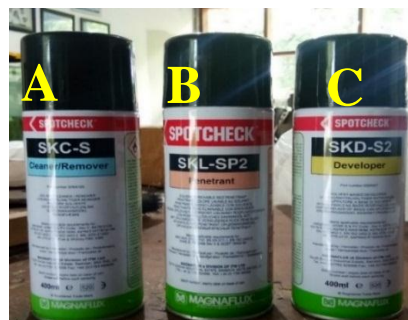
Gambar 3. Cleaner / Remover (A), Liquid Penetrant (B), Developer (C)
