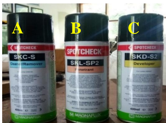
Gambar 6. Cleaner / Remover (A), Liquid Penetrant (B), Developer (C)
