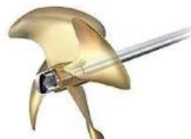
Gambar 3. Propeller biasa tipe fixed pitch propeller
